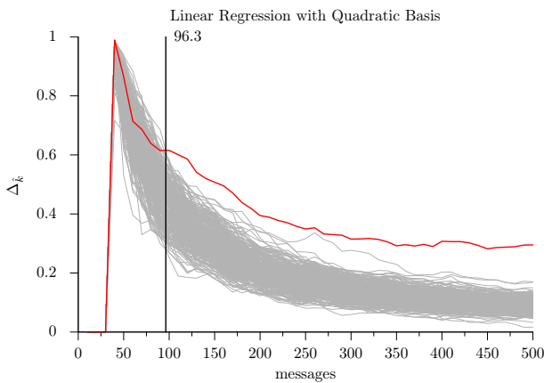
Fig. 8: Evolution of the distinguishing value (y-axis) with the number of messages (x-axis) for all key candidates for linear regression with quadratic basis. The curve of the real key used in the device is plotted in red.
